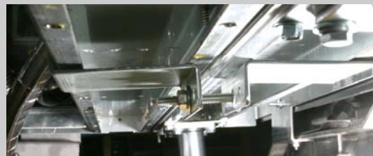
Figure 4: Attach the provided brackets on either side of the center caster. Insert the bolts and draw the fryer components together, aligning the caster plate holes with the mounting points. (View is from bottom of fryer.)
