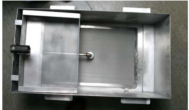
Crumb screen properly placed in filter pan.
