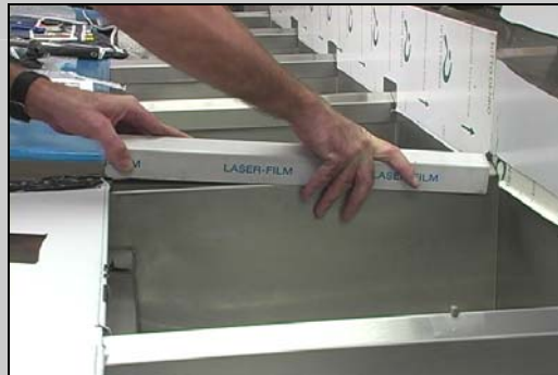
Figure 9: Place joiner strip which connects the frypots.
